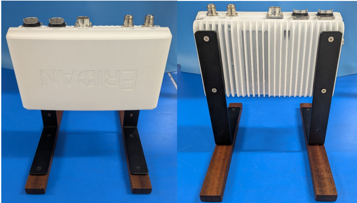
RU mounted on the provided stand (front and back) for optimal airflow.
